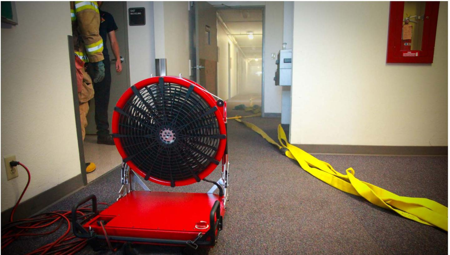
***With a Jet Approach to PPV the BlowHard BH-20 is able to build more pressure than the conventional approach resulting in increased ventilation. The BH-20 is capable of air movement equivalent to fans rated 15,000 CFM or higher in real-world conditions.***
